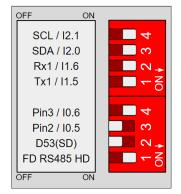
**4. SCL/I2.1:** Choosing between SCL or the input I2.1. If this switch is ON, it enables the I2.1 input and disables the SCL. If this switch is OFF, it enables SCL and disables I2.1.
