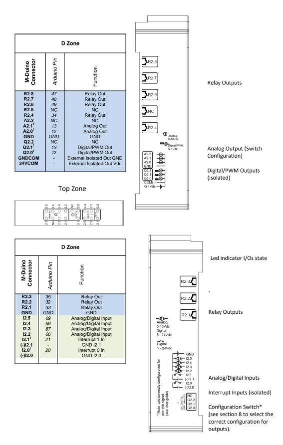
See section 8 to select suitable switch configuration for enable these connections.
