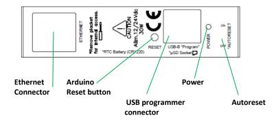
\*NOTE: Autoreset. Arduino mega has auto reset when using serial communication code. Set switch to OFF when using serial communication. When uploading code to Arduino Mega set switch to ON.
