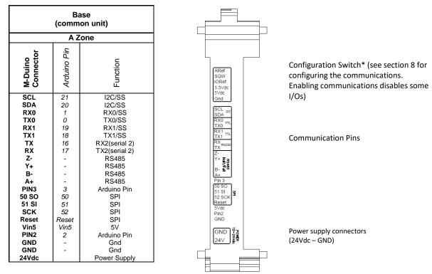
SS: Chip Select pins. These pins can act as TTL, so they can work for the Chip Select pin of any device.
